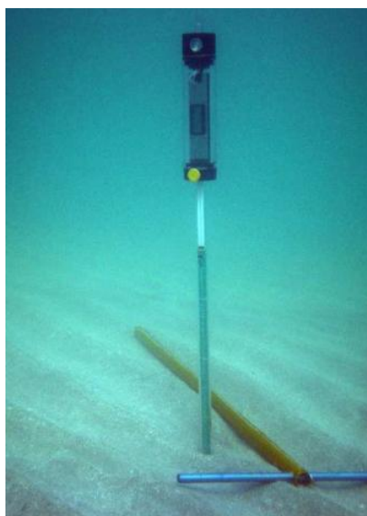
Figure 4.4. Example of SediMeter installation (Lindorm 2009a)
